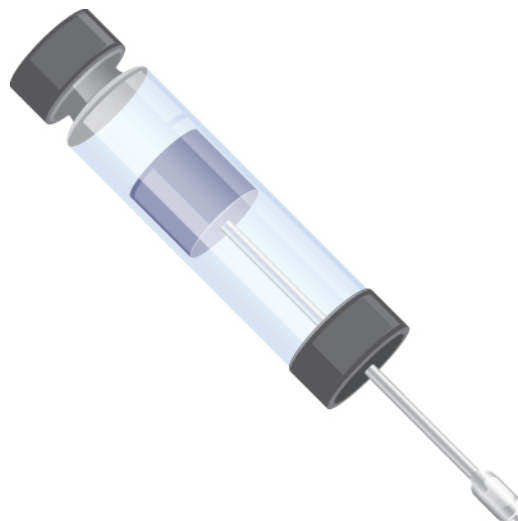
Figure 7.5 A dashpot is a pneumatic cylinder that dampens the motion of an oscillating system.
